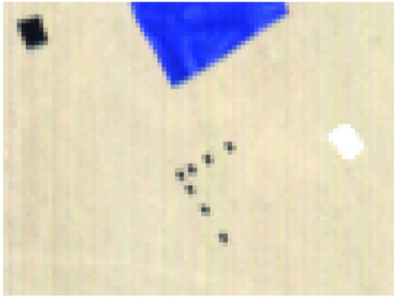
Fig. 26. Raw PRISM image of 30 cm square tiles (seven tiles in the middle of the frame) placed on the dry lakebed surface, adjacent to the radiometric calibration target. The corner tile is separated by 30 cm from each of its neighbors.
